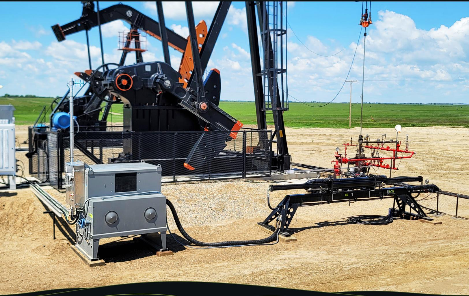
**IJACK EGAS** AUTOMATED STAND ALONE WET CASING GAS COMPRESSION SYSTEM IS ENGINEERED TO OPTIMIZE WELL PERFORMANCE BY RELIEVING CASING PRESSURE AND ALLOWING UNRESTRICTED PRODUCTION INFLOW FROM THE FORMATION. WITH ITS USER-FRIENDLY INTERFACE AND ADVANCED AUTOMATION CAPABILITIES, IJACK™ EGAS ALLOWS YOU TO SET YOUR DESIRED CASING PRESSURE AND WATCH AS IT AUTOMATICALLY ADJUSTS ITS PARAMETERS TO ACHIEVE YOUR PRODUCTION GOALS.
